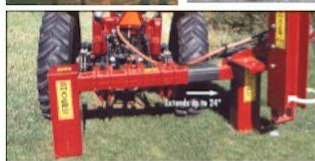
Hydraulic post driver—either centre mounted or offset behind tractor. Also available mounted on Weidemann loader
